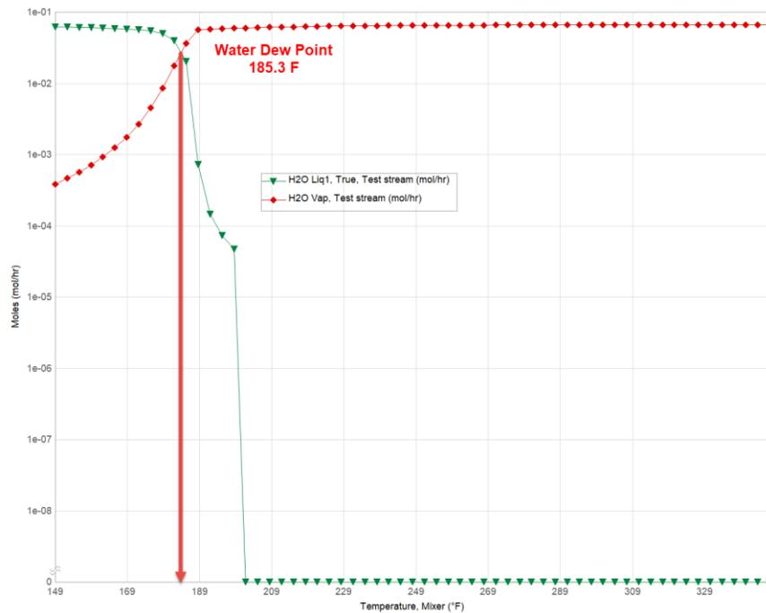
Figure 2. Detecting the water dew point
