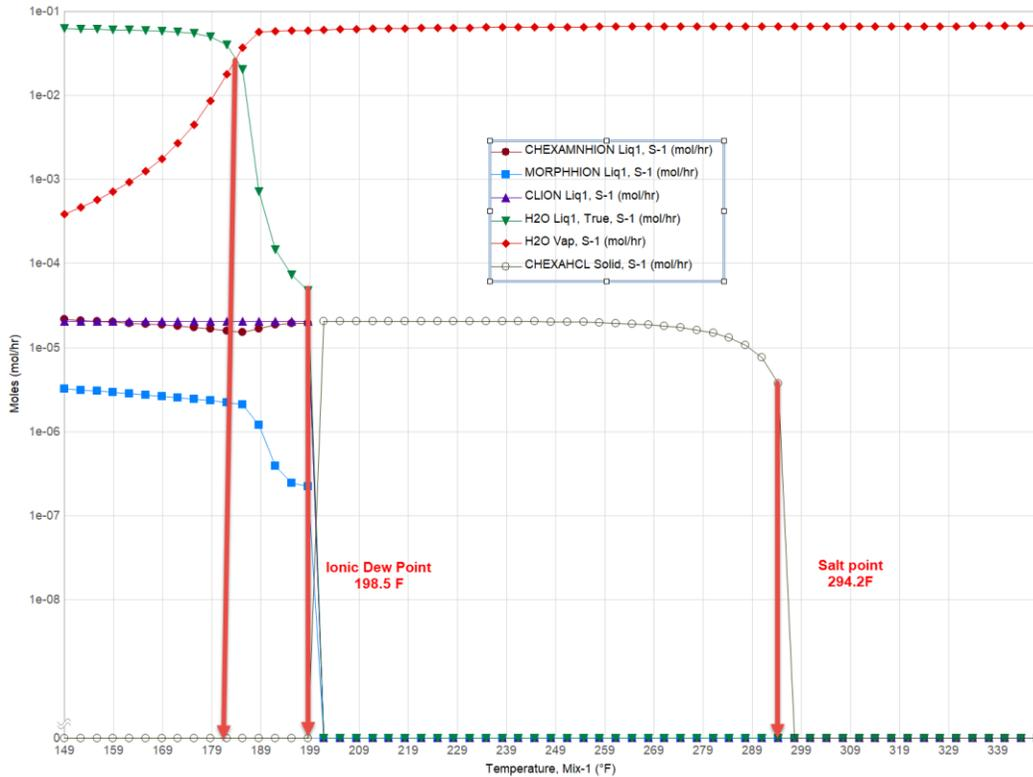
Figure 5. Composite salt point, ionic dew point, and water dew point
