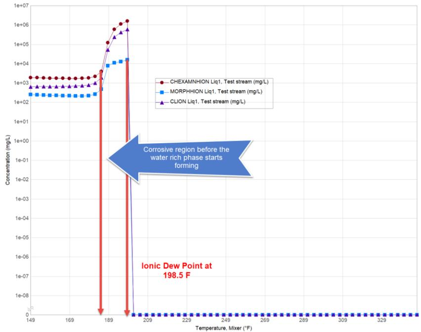
Figure 3. Detecting the ionic dew point of morpholine
