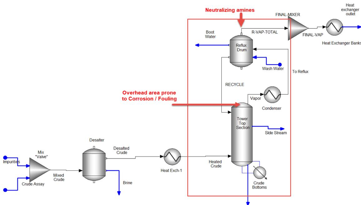
Figure 1. CDU and overheads simulation
