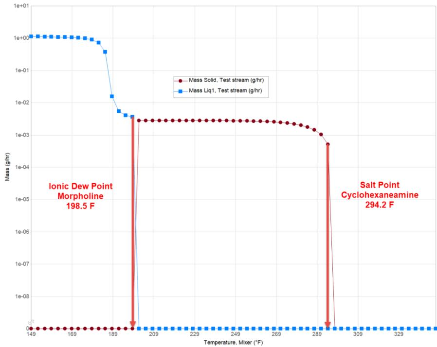
Figure 4. Detecting the salt point of cyclohexaneamine
