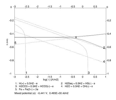
Figure 10. Predicted current density - potential relationship and partial cathodic and anodic processes for Fe in a CO<sub>2</sub>+H<sub>2</sub>S system at 30 °C under static conditions. The partial pressure of H<sub>2</sub>S is 0.23 atm and the total pressure is 1 atm.
