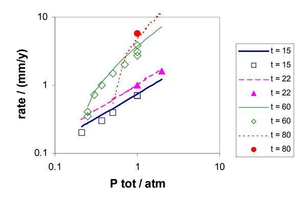
Figure 5. Corrosion rate as a function of total pressure for carbon steel in a 0.1 % NaCl solution in the presence of CO<sub>2</sub> at various temperatures. The lines have been obtained from the model and the symbols denote the data of de Waard and Milliams<sup>1</sup> for X-52 steel.
