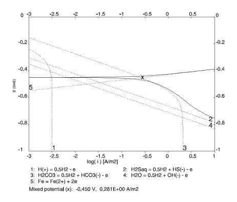
Figure 9. Predicted current density - potential relationship and partial cathodic and anodic processes for Fe in a  $CO_2+H_2S$  system at 30 °C under static conditions. The partial pressure of  $H_2S$  is 0.01 atm and the total pressure is 1 atm.
