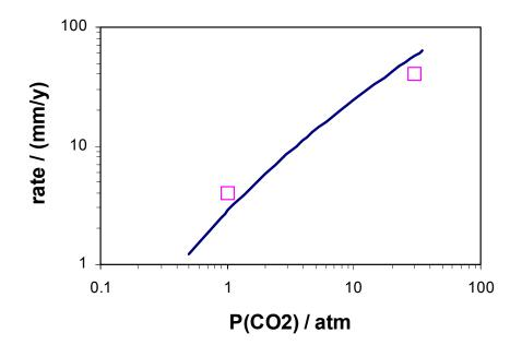
Figure 6. Corrosion rate as a function of pressure for carbon steel in synthetic seawater in the presence of  $CO_2$  at 60 °C. The line has been obtained from the model and the symbols denote the data of Ikeda et al.<sup>37</sup>
