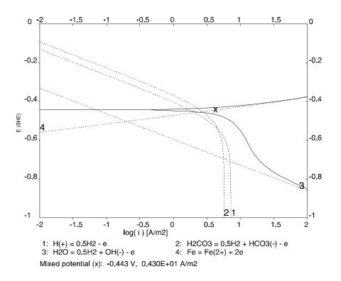
Figure 3. Predicted current density - potential relationship and partial cathodic and anodic processes for carbon steel in a 1 % NaCl solution in the presence of CO<sub>2</sub> at 1 bar and 60 °C under the conditions of pipe flow with a velocity of 2 m/s and pipe diameter of 1.5 cm. The natural pH of the system is 4.04.
