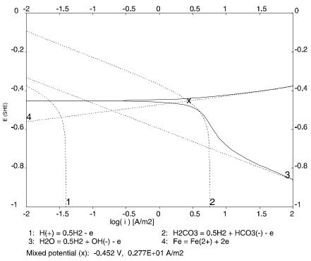
Figure 4. Predicted current density - potential relationship and partial cathodic and anodic processes for carbon steel in a 1 % NaCl solution in the presence of  $CO_2$  at 1 bar and 60 °C under the conditions of pipe flow with a velocity of 2 m/s and pipe diameter of 1.5 cm. The pH of the system has been adjusted to 6 by adding NaOH.
