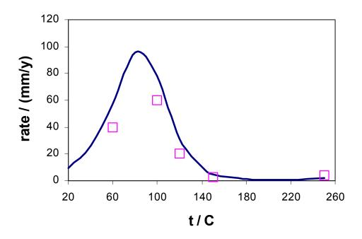
Figure 7. Corrosion rate as a function of temperature for carbon steel in synthetic seawater. The CO<sub>2</sub> pressure is 30 bar at room temperature. The line has been obtained from the model and the symbols denote the data of Ikeda et al.<sup>37</sup>
