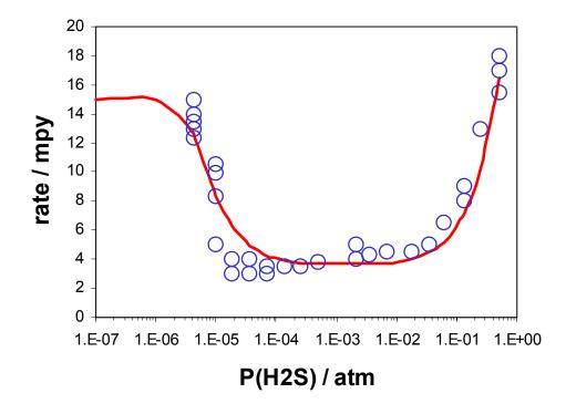
Figure 8. Corrosion rate as a function of H<sub>2</sub>S partial pressure for Armco iron at 30°C. The total pressure (CO<sub>2</sub> and H<sub>2</sub>S) is 1 atm. The line has been obtained from the model and the symbols denote the data of Greco and Wright.<sup>17</sup>
