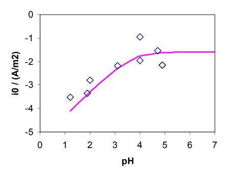
Figure 1. Representation of the exchange current density for iron dissolution at different pH values. The symbols denote the experimental data of Bockris et al.<sup>29</sup>.
