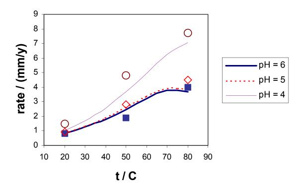
Figure 2. Corrosion rate for carbon steel in a 1 % NaCl solution in the presence of  $CO_2$  at 1 bar under the conditions of pipe flow with a velocity of 2 m/s and pipe diameter of 1.5 cm. The lines have been obtained from the model and the symbols denote the data of Nesic et al.<sup>12</sup> for X-65 steel.
